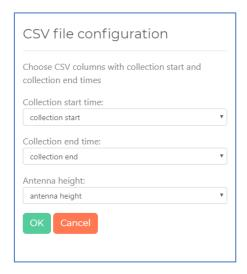
Click "Batch process" or you can manually process. Export CSV file. Latitude, longitude and elevation cloumns show the coordinates of the center point of corrected values at each GCP. Save them to a separate CSV file together with station id as GCP coordinates
